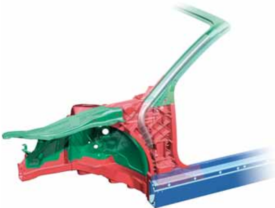
Reinforced A-post with reinforced windscreen frame and door sills
