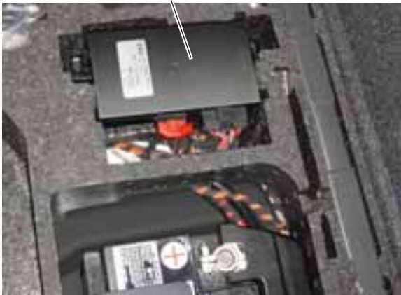
Convertible top operation control unit J256
