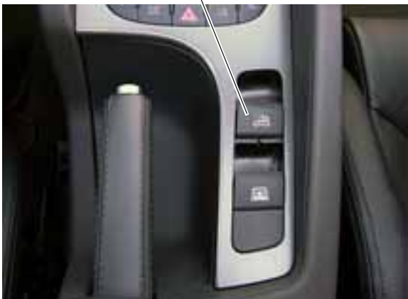
Convertible top operating switch E137
