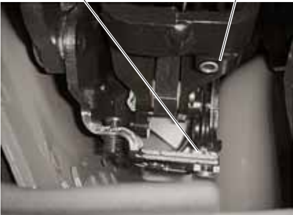
Convertible top front switch F202
