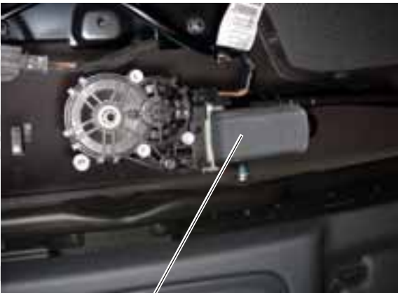
Convertible top lock motor V223
