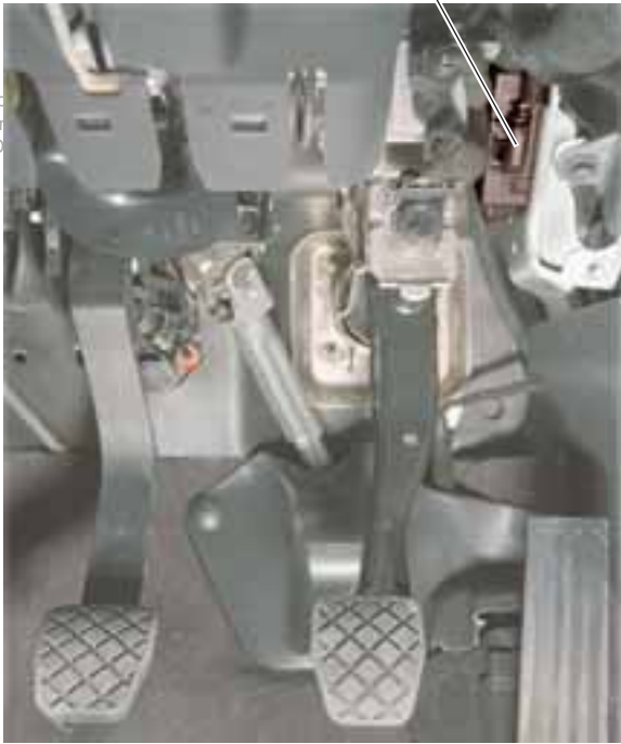
Data bus diagnostic interface J533
