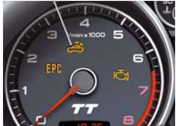
Convertible top operation warning lamp K215
