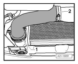
Remove bolt -1- and take out intake connecting pipe from below.
