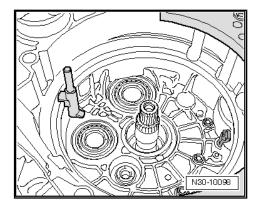
Install multiple clutch in clutch bell housing (turn and move up and down as required), at the same time keeping the drive plate pressed into the outer plate carrier with both thumbs -arrows-.
