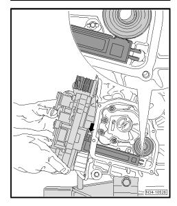
Tighten bolts for mechatronic unit for direct shift gearbox -J743-; note correct tightening sequence <u>⇒ page 81</u>.
