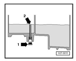
The gear oil that has collected in the overflow pipe -arrow 2will drain off first.
