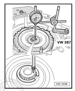
For 2nd measurement, apply tip of dial gauge to hub of inner plate carrier as shown in illustration.
