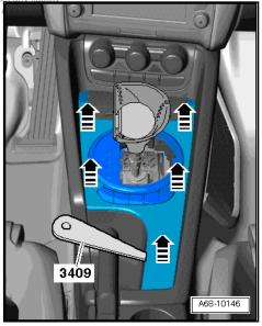
Remove bolts -arrows- and detach trim for selector lever boot -1- together with selector lever display illumination bulb -L101- .
