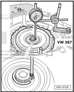
Remove provisionally fitted circlip (2 mm) and fit new circlip with thickness as calculated above.
