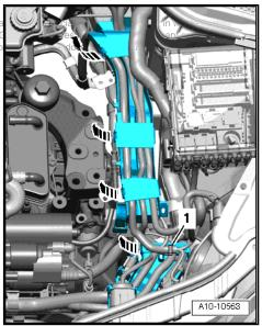
Remove bolts -1- and detach gearbox mounting -A-.
