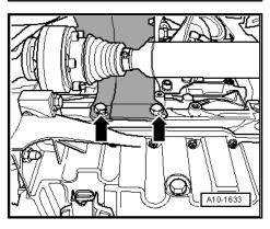
Remove bolt -arrow- and detach flange shaft (right-side) from gearbox.
