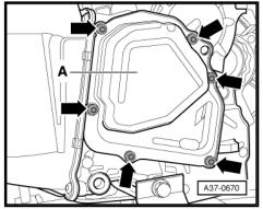
Remove bolts -arrows- and detach cover for gear oil pump -1-.
