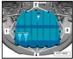
Remove noise insulation (left-side) -arrows-.
