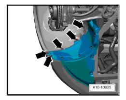
Remove bolts -arrows- and detach cover for gear oil pump -A-, allowing remaining gear oil in cover to drain off into used oil collection and extraction unit -V.A.G 1782- .
