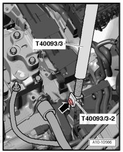
Insert square bars -T40091/1- with connecting pieces -T40093/4- into connecting pieces -T40091/3- and supports -T40093/3- as illustrated.
