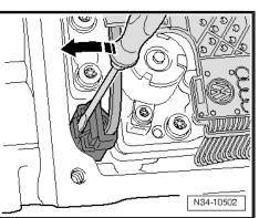
Release wiring leading to -G182- and -G509- from retaining tabs on mechatronic unit -arrows I and II-.
