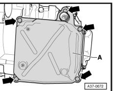
Remove noise insulation (left-side) -arrows-.
