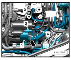
Clamp off coolant hoses at gearbox oil cooler with hose clamps -3094- and disconnect hoses from gear oil cooler -A-.
