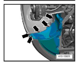
Remove frame for noise insulation -arrow-.
