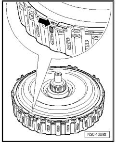
Pry out old circlip -2- using a screwdriver -1- -arrow-.
