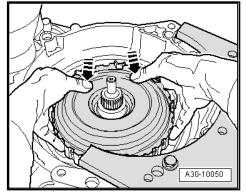
Have a second mechanic hold the retaining pin -T10303- as illustrated until the clutch end cover is installed.
