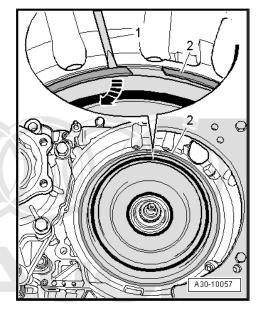
Working through aperture for starter motor, pry out and detach ht. Copy clutch end cover -2- using a screwdriver -1- or other suitable uthorised lever -arrow-.
