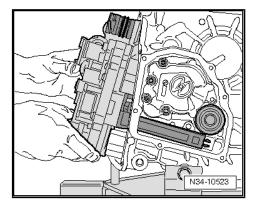
Put down the mechatronic unit correctly.
