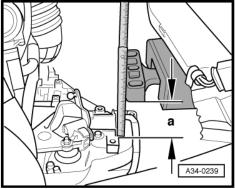
To remove the direct shift gearbox 02E, set up gearbox support -3282- with adjustment plate -3282/42A- and place on engine and gearbox jack -V.A.G 1383 A-.
