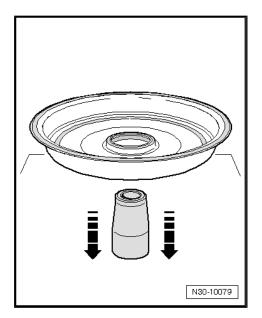
Fit assembly sleeve -T10302- over end of multiple clutch shaft.
