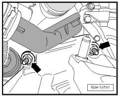
Secure bracket -T10338- to vacant tapped hole at rear left of engine.
