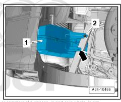
Protected by copyright. Copying for private Remove noise insulation frame -arrow=septiteReps Graths50 d by AUDI AG. A with respect to the correctness of information of the correctness of the correctness
