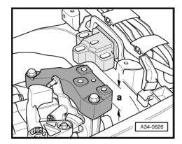
Unbolt gearbox bracket from gearbox -arrows-.
