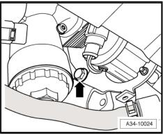
Unscrew engine/gearbox securing bolt -arrow- located next to bevel box -C-.
