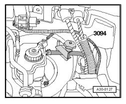
If a pipe/hose assembly is installed between clutch master cylinder and slave cylinder, clamp off hose -A- using hose clamp -3094- .
