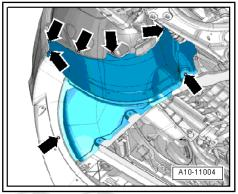
Unscrew bolt -2- and disconnect air duct for gearbox cooling -1- (-arrow-).
