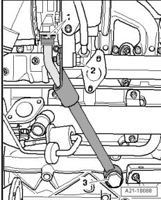
Remove bolts -arrows 1, 2, 3- and detach bracket for bevel box.
