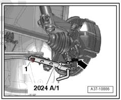
Slacken bolts -1- and remove bolts -2-.
