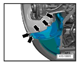
Remove noise insulation frame -arrow- ⇒ Rep. Gr. 50.
