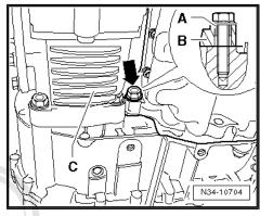
To remove gearbox "02Q" set up gearbox support -3282- with adjustment plate -3282/33- .
