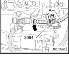
Unbolt gearbox bracket from gearbox -arrows-.
