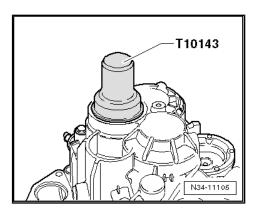
Secure sealing cap with circlip -A-.
