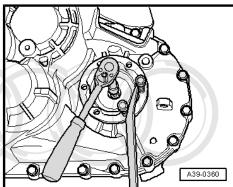
Remove bolts -B- securing gearbox housing from inside clutch housing.
