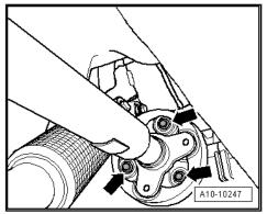
Push engine/gearbox assembly forward slightly (towards front end) and then pull propshaft off bevel box.
