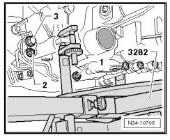
Separate gearbox from engine and pivot upwards at differential end. Guide output flange -C- on gearbox past propshaft -A- and front exhaust pipe -B-. Rotate output flange if neces-
