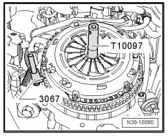
To prevent the pressure plate from becoming distorted during installation (causes clutch grab when driving off), always adhere to the following procedure when installing the pressure plate:
