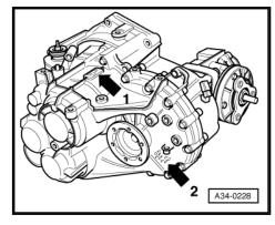
Manual gearbox 02Q, four-wheel drive -arrow-
