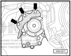
Heat shield for drive shaft (right-side) for vehicles with 2.0 ltr. TDI engine: tightening torque  $\,$
