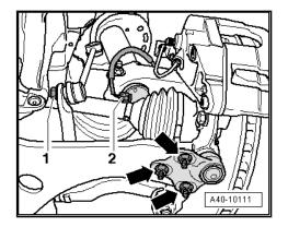
Unbolt heat shield for drive shaft (right-side) from bevel box -arrows-.
