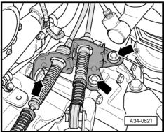
Remove top engine/gearbox securing bolts -1-.
