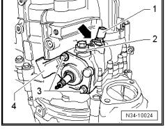
Remove bolt securing flange shaft (left-side). To do so, screw two bolts into flange and counterhold flange shaft with suitable
