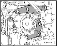
Turn gearbox upwards at differential end. Guide output flange -C- on gearbox past propshaft -A- and front exhaust pipe -B-. Rotate output flange if necessary.
