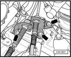
Unscrew top engine/gearbox securing bolts -arrows-.
