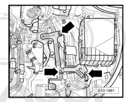
Detach securing clip -1- and pull cable end-piece off pin.
