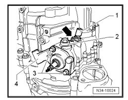
Install flange shaft together with spring, thrust washer and tapered ring.
