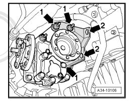
Unscrew bolts -arrow-, detach oil return line from turbocharger and press to right side by copyright. Copying for private or commercial purposes, in part permitted unless authorised by AUDI AG. AUDI AG does not guarantee or with respect to the correctness of information in this document. Copyright
