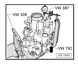
Press in tapered roller bearing outer race together with the correct shim (in example 1.65 mm). Support gearbox housing with thrust piece -2050- directly below bearing mounting.
