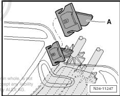
Attach cable support bracket to gearbox -arrows-. Tightening torque ⇒ page 68
