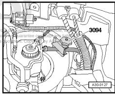
If a pipe/hose assembly is installed between clutch master cylinder and slave cylinder, clamp off hose -A- using hose clamp up to 25 mm -3094- .
