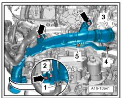
Detach securing clip -arrow 1- and pull cable end-piece off pin.
