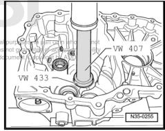
Fit gearbox housing and tighten bolts -A- and -B- diagonally to correct torque.
