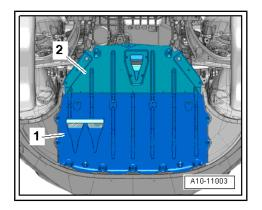
Remove noise insulation (left and right) -arrows-.
