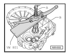
Press in tapered roller bearing outer race together with the correct shim (in example 1.75 mm). Support gearbox housing with thrust piece -2050- directly below bearing mounting.
