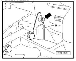
Press engine/gearbox assembly towards bulkhead, taking care to guide pin on bevel box into propshaft flange.
