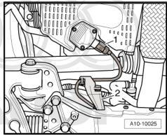
Unbolt bracket for exhaust system -arrows- and pull bracket rised by
