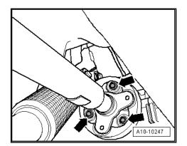
Push engine/gearbox assembly forward slightly (towards front end) and then pull propshaft off bevel box.
