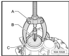
Detach circlip -C- from input shaft grooved ball bearing as follows:
