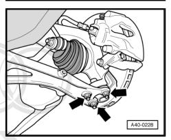
Swivel suspension strut (right-side) outwards and support with extension -2024 A /1-, as shown in illustration.
