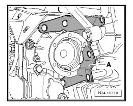
Screw in and tighten bottom engine/gearbox securing bolts -1 ... 3- first, then remaining securing bolts ⇒ page 120 .
