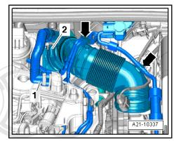
Lift retaining clips -arrows- and disconnect coolant hoses from heat exchanger.
