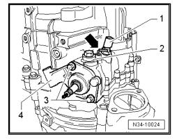
Remove bolt securing flange shaft (left-side). To do so, screw two bolts into flange and counterhold flange shaft with suitable lever.
