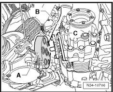
If necessary, install bracket for bevel box -A-.
