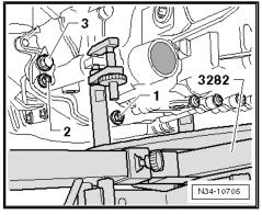
Lubricate bearings and moving surfaces of gate relay lever -1- with grease -G 000 450 02- .
