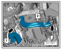
Remove bolts -1, 2, 3- and detach bracket for bevel box.
