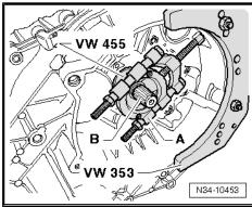
Remove reverse gear selector fork -A-
