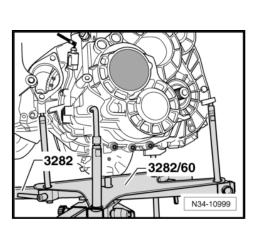
Screw pin -3282/34- into hole for bolt securing pendulum support to gearbox.
