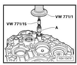
Driving in selector rod bearing bush -A- to stop
