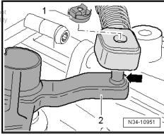
Unscrew bolts -arrows-, remove cable support bracket from gearbox and tie up on left side.
