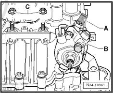
Drive sealing cap into gearbox housing as far as stop of thrust piece -T10042- .
