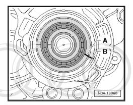
Install circlip -1- for input shaft grooved ball bearing.
