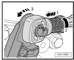
Detach securing clip -1- for gear selector cable from gearbox selector lever -2- and pull selector cable off pin -arrow-.
