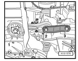
Remove bolts -1- and -2- and detach bracket for starter catalytic converter.
