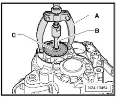
Remove circlip -C- from grooved ball bearing of input shaft as follows:
