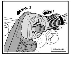
Detach securing clip -1- for gear selector cable from gearbox selector period by 2 points of policy and policy selector cable from gearbox selector period of the selector cable from gearbox sele
