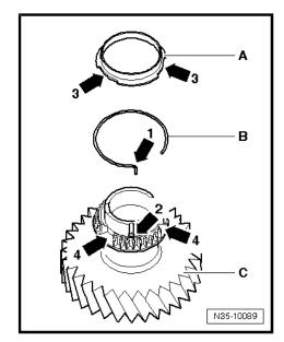
Then carefully press stop ring -A- onto selector gear. Keep spring compressed -arrows- while pressing on stop ring.
