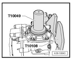
Pack space between sealing lip and dust lip half-full with sealing grease -G 052 128 A1-.
