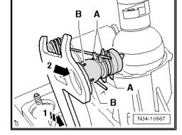
Insert selector housing with gear lever guide in larger recess -arrow- in thrust block -T10083- .
