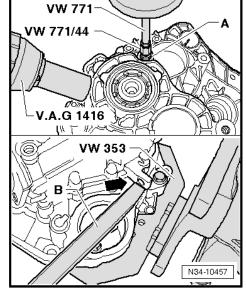
Remove splitter -A- and installing sleeve -VW 455- from input shaft -B-.
