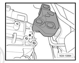
Set up gearbox support -3282- with adjustment plate -3282/60to remove gearbox "0A6".
