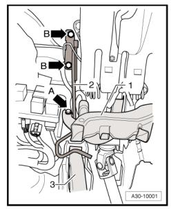
Unbolt clutch pedal -1- from mounting bracket -3-. To do this, remove nut -2- and pull out bolt -5-.
