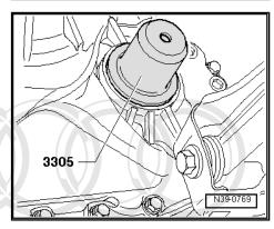
Pack space between sealing lip and dust lip -arrow- half full with sealing grease -G 052 128 A1- .
