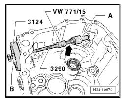
Driving in selector shaft bearing bush -A- to stop of tool
