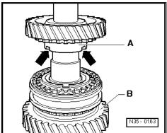
Pressing on tapered roller bearing inner race for bearing in gearbox housing and fitting circlip
