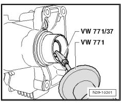
Lever out stub shaft oil seal on drive shaft side.
