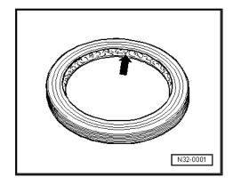
Drive in oil seal on gearbox side as far as stop.
