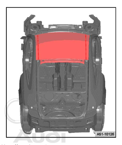
Remove remaining material on roof frame using compact angle grinder -VAS 5167
