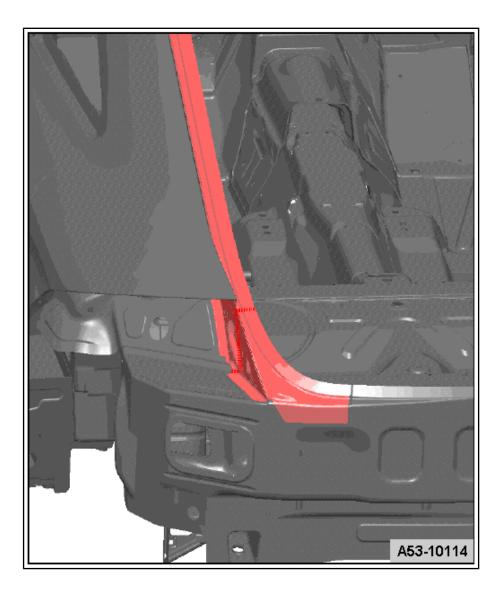
Make separating cuts as shown using pneumatic sabre saw -V.A.G 1523A- .
