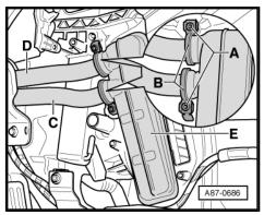
Check position of both clips -B- after tightening bolts -A-. Clips must completely surround flange at heat exchanger and coolant pipe and not make contact with other components.
