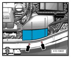
Screw out the bolts -arrows- and detach the air duct (vehicles with 6-cylinder engine only).
