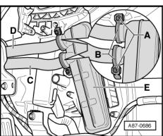
Fit the bolt -A- at the connecting flange -B- (in doing so, make sure the bolt really is screwed in at the intended attachment point).
