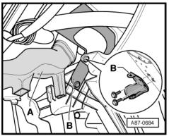
Remove the holder -B- ⇒ General body repairs, interior; Rep. Gr. 68.
