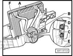
On inserting evaporator -A- in bottom part of evaporator housing and on assembling the two halves of the housing, take care not to damage seal -F-.
