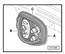
Take out the air conditioner unit (heater) -A- towards the passenger's side.
