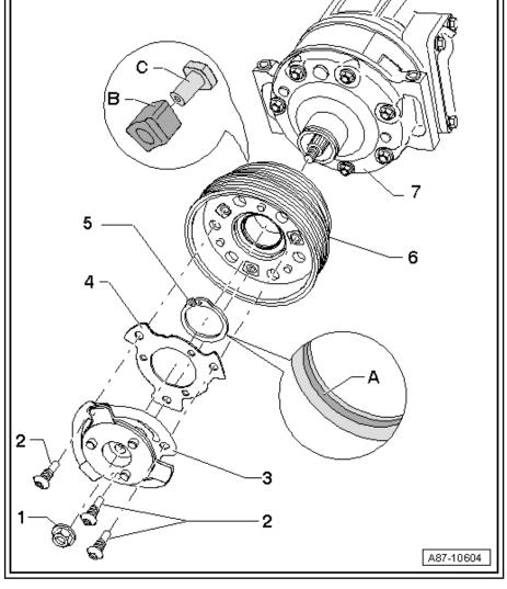
□ Apply locking fluid when fitting the bolts (e.g. D 000 600 A2) ⇒ Electronic parts catalogue.
