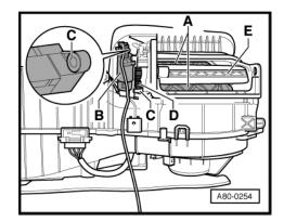
Insert the air flow flap control motor -V71- -B- in the direction opposite to the arrow in the mounts -C- and position it on the gear wheel -D-.
