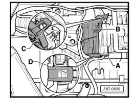
Detach the control motor -A- from the intake housing.
