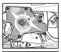
Mark positions of coolant hoses -A- and -B-.
