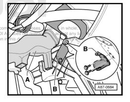
Remove the 4 bolts -A- and detach cover -B-.
