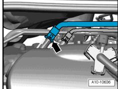
Remove the components impeding access to the coolant hoses -A- and -B- in the engine compartment ⇒ Engine, mechanics; Rep. Gr. 13.
