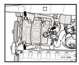
Before securing the air conditioner compressor, check the position of both dowel sleeves -arrows- in the holder or air conditioner compressor.
