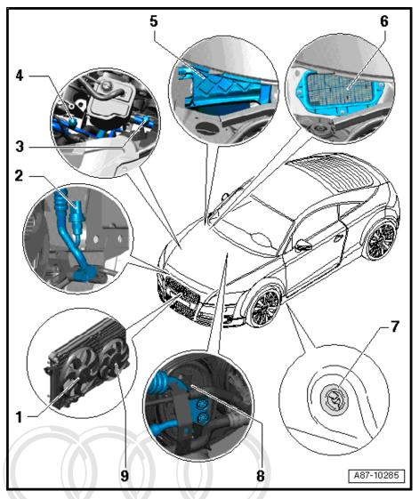
switches e.g. the radiator fan -V7- and the radiator fan 2 -V177- (directly via the radiator fan control unit -J293- ) infinitely to the desired output (depending on the engine type). ⇒ "Guided fault-finding" function of vehicle diagnostic, testing and information system VAS 5051 and ⇒ Current flow diagrams, Electrical fault finding and Fitting locations.
