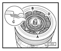
Insert the drive plate -C- in the rubber elements -D- (refer to illustration above) until it makes contact with the shaft of the air conditioner compressor -B-.
