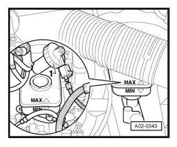
Use extraction hose included in brake filling and bleeding equipment -VAS 5234- to extract as much brake fluid as possible.
