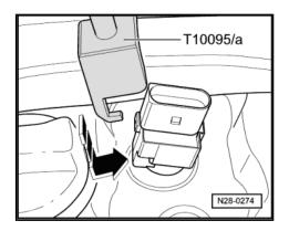
Note installation position of ignition coils with output stage relative to connectors before you remove the coils -arrows-.
