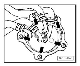
Remove filter element -1- and seals -2 and 3- from filter housing -4-.
